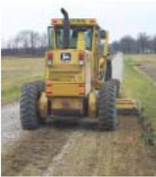
The RotoGrader is easily side shifted with the blade to cut and pulverize road shoulders in a single pass.
